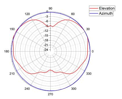
Frequency: 4.9GHz Max Gain: 4dBi
