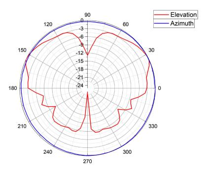
Frequency: 5.8GHz Max Gain: 4dBi
